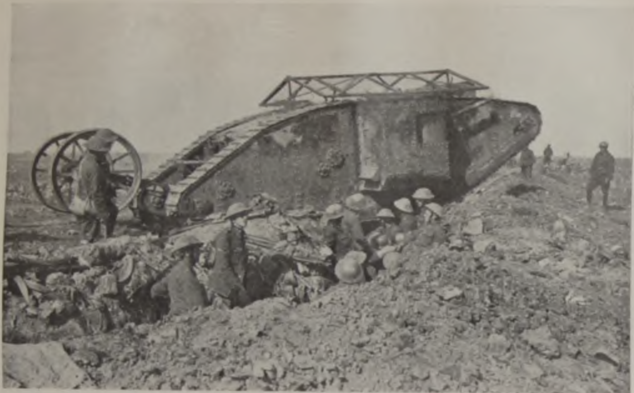
THE COMING OF THE TANKS. The tank first saw action on September 15, 1916. There were two types of this machine - the male, equipped with two 6-pounder guns and a machine gun, and the female, armed with machine guns only. Above is shown a Mark I male tank on the Somme battlefield.
