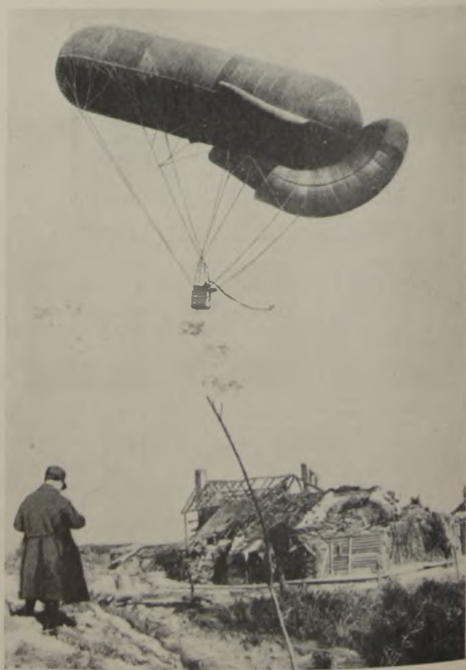
A BELGIAN OBSERVATION BALLOON. Balloons were used by the intelligence department for reconnoitering over the lines. The type here shown possessed remarkable stability, and could remain aloft during a gale. The observers, whose main work was to search the terrain for German artillery positions, were provided with parachutes, so that in case of attack by aeroplane they could reach the ground in safety.
