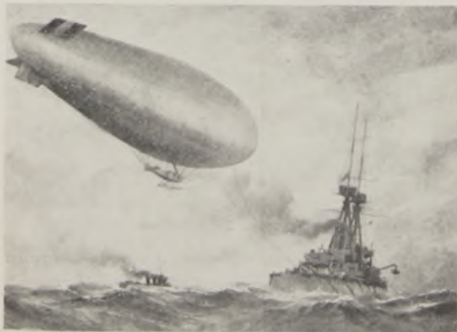
British blimp, or naval observation airship, being towed by warship against a strong headwind. The blimp was a non-rigid type used by the Admiralty for scouting purposes.
