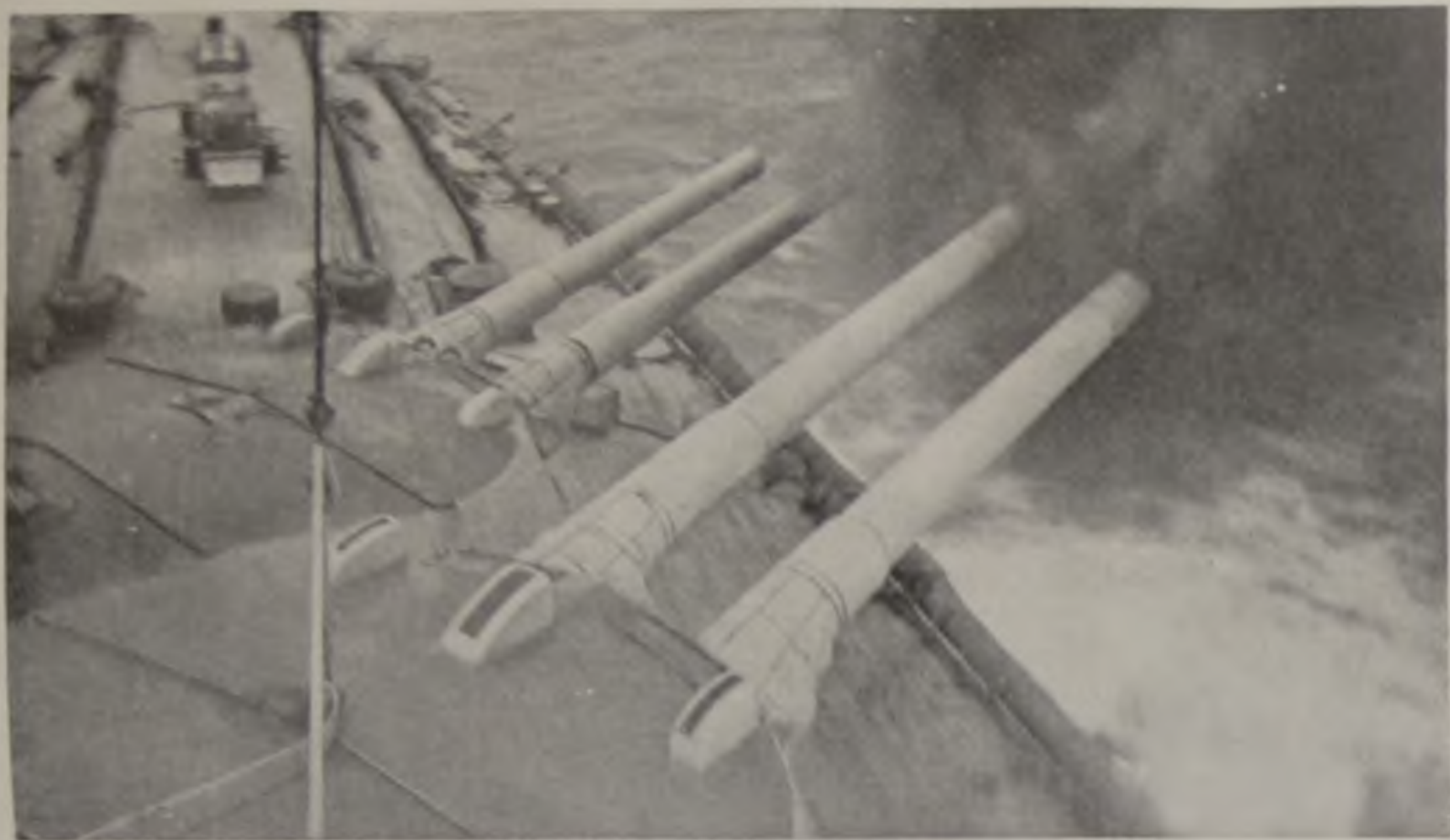
THE GREAT GUNS SPEAK. This war-time photograph shows an actual discharge of a salvo of 13.5-inch guns from a British battle cruiser. With two exceptions, all British battle cruisers after the Indomitable class carried eight 13.5 guns a simultaneous discharge of four guns usually constituting a salvo
