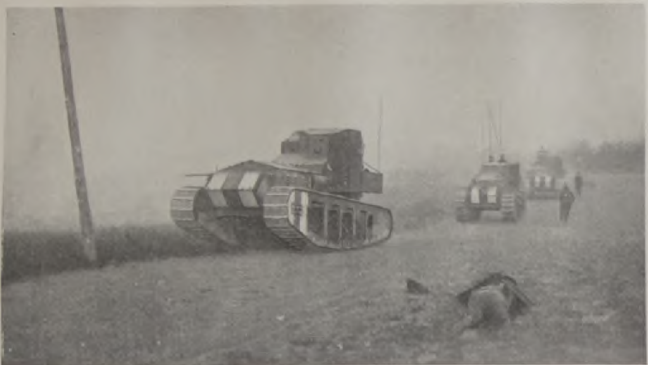
WHIPPET TANKS IN ACTION. Besides the heavy tanks in 1918 a medium-sized machine known as the medium A, or whippet, tank was introduced as a "cavalry" or pursuit weapon. It could move at from eight to ten miles an hour and its crew consisted of three men. In the above photograph three of these machines are seen advancing to attack during one of the great battles of August, 1918.
