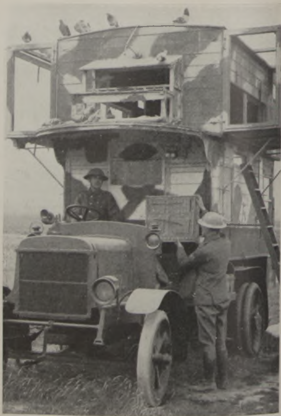
A FIELD LOFT FOR PIGEONS. Pigeons are invaluable to armies, and during the Great War performed very varied tasks. In Plates 42-43 they are seen in action on land and sea. This photograph shows a pre-war London omnibus turned into a motor loft for field service.
