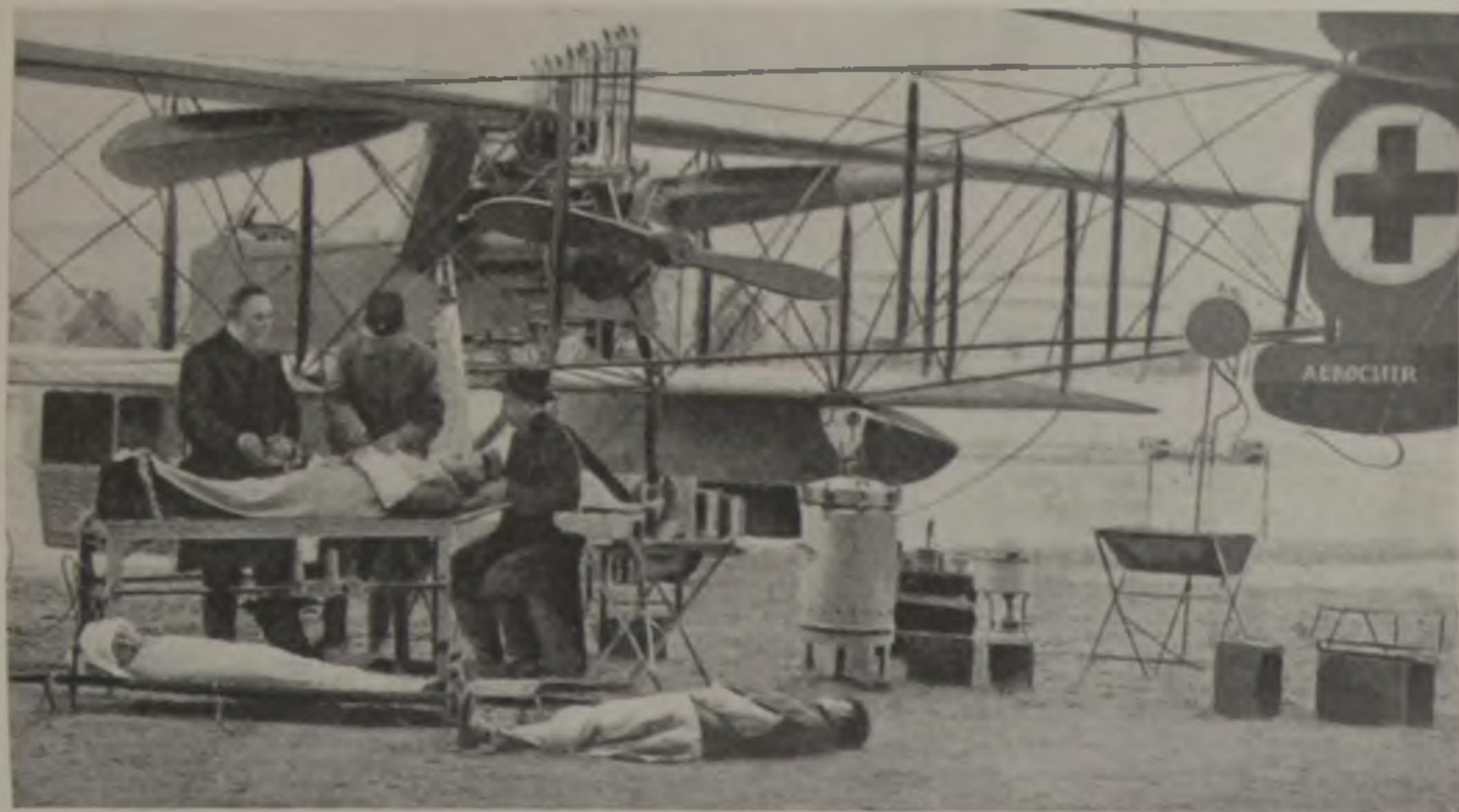
RED CROSS AMBULANCE OF THE AIR. A remarkable war-time invention was the French aeroplane the "Aerochir," designed for medical service. The staff are X-raying one patient, while others await attention. This aeroplane had compartments for surgical instruments and materials and sterilising apparatus and dressings.
